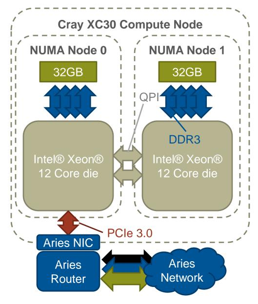
An Ivybridge XC30 blade has two sockets, each with 12 Intel Cores. Each Intel core is termed a "Compute Unit".
