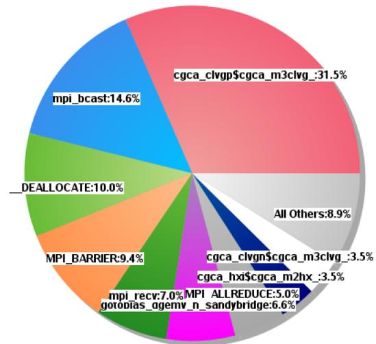
Fig. 14. Profiling function distribution with `cgca_gcupdn` and `cgca_pfem_map` at 7200 cores.
