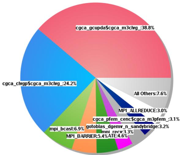
Fig. 9. Profiling function distribution for ParaFEM/CGPACK MPI/coarray miniapp with all-to-all routine `cgca_gcupda` at 7200 cores.
