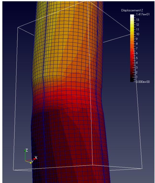
Fig. 5. The distorted FE mesh at the end of the CAFE simulation, with the axial displacement contours.
