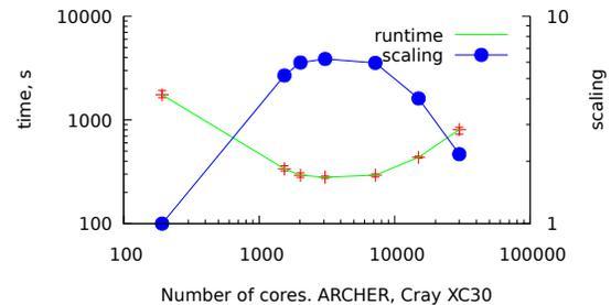
Fig. 8. ParaFEM/CGPACK MPI/coarray miniapp scaling on ARCHER XC30 for a 3D problem with 1M FE and 800M CA cells.
