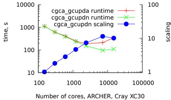
Fig. 13. Runtimes and scaling for ParaFEM/CGPACK MPI/coarray miniapp with the nearest neighbour, `cgca_gcupdn`, and all-to-all, `cgca_gcupda`, algorithms.
