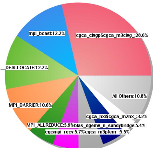
Fig. 11. Raw profiling data for ParaFEM/CGPACK MPI/coarray miniapp with the nearest neighbour routine `cgca_gcupdn` at 7200 cores.
