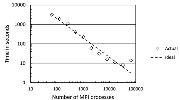
Fig. 6. ParaFEM scaling for a 3D transient flow explicit analysis. Reproduced from [7].
