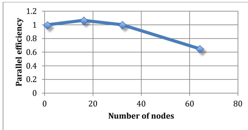
Figure 3: Scaling of TPLS 3 for 11 Million Point Domain
