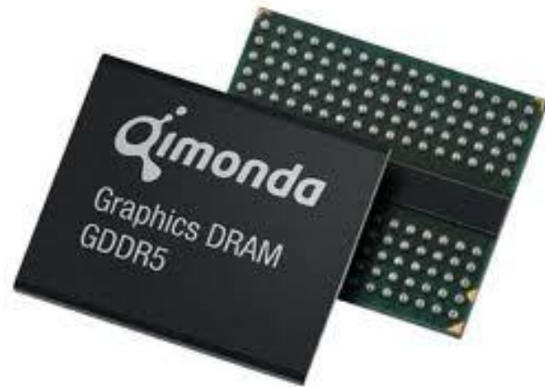
GPUs and Xeon Phi use Graphics DRAM
