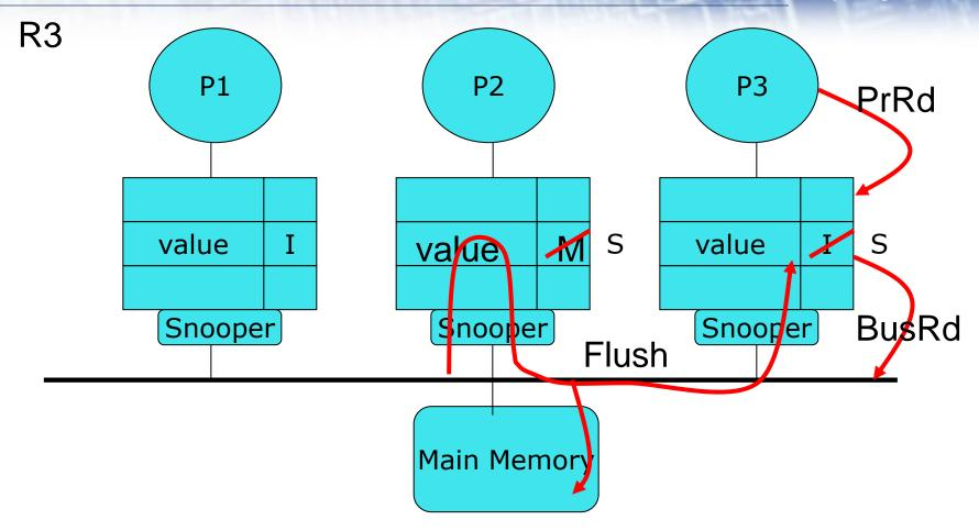
P3 wants to read the value. Its cache does not have a valid copy, so it places a BusRd on the bus. P2 has a modified copy, so it flushes the data on the bus and changes the status of the cache data to shared. The flush cancels the memory access and updates the data in memory as well.
