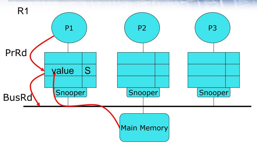
P1 wants to read the value. The cache does not have it and generates a BusRd for the data. Main memory controller provides the data. The data goes into the cache in the shared state.
