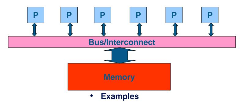
IBM servers, Sun HPC Servers, Fujitsu PrimePower, multiprocessor PCs
