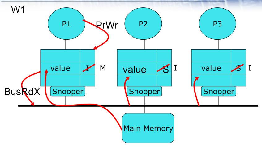
P1 wants to write to its cache. The cache places a BusRdX on the bus to gain exclusive access and the most up-to-date value. Main memory is not stale so it provides the data. The snoopers for P2 and P3 see the BusRdX and invalidate their copies in cache.
