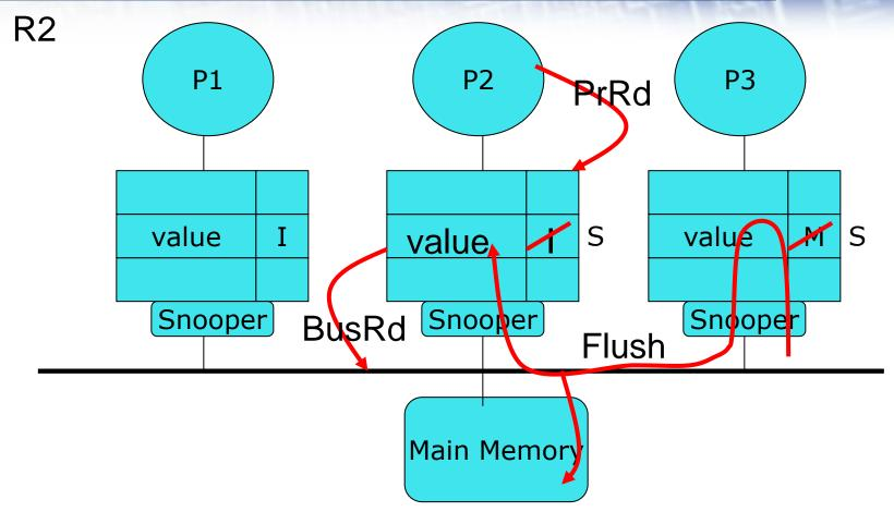
P2 wants to read the value. P3's cache has the most up-to-date copy and will provide it. P2's cache puts a BusRd on the bus. P3's cache snoops this and cancels the memory access because it will provide the data. P3's cache flushes the data to the bus.
