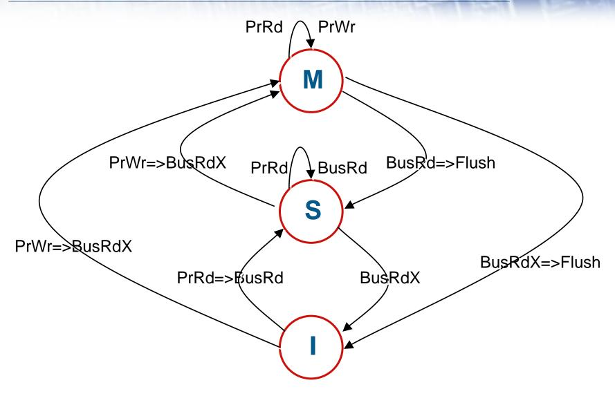
A=>B means that when action A occurs, the state transition indicated happens, and action B is generated
