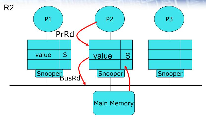
P2 wants to read the value. Its cache does not have the data, so it places a BusRd to notify other processors and ask for the data. The memory controller provides the data.
