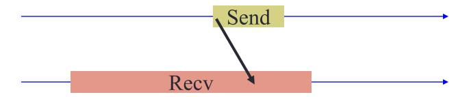
• If blocking receive is posted before matching send, then the receiving task must wait until the data is sent.
