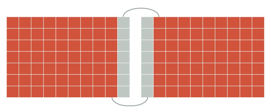
Halos transferred via MPI\_Sendrecv
